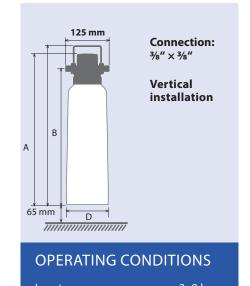
Input pressure: 2–8 bar Water temperature: 4-30 °C Ambient temperature: 4-40 °C
