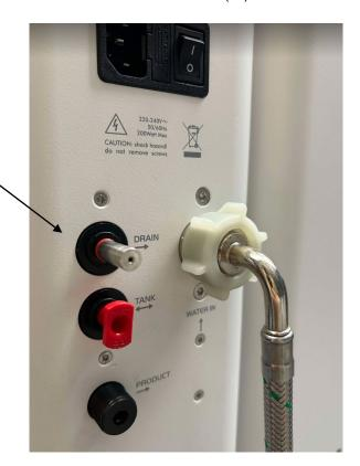
The Drain elbow (3) can now be mounted on the Concentrate Restrictor (10).
