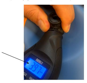
The factory-set (default) pressure is approximately 4 bars. Deflate the tank to 1 bar before use.
