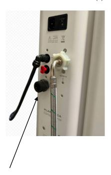
Mount the outlet water hose (13) on the reduction (9) on the
