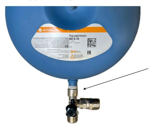
Note: The auto flush valve (18) is only connected, so that it is possible to drain the buffer tank (12) if needed. Remember to keep the auto flush valve closed when the system is operating.
