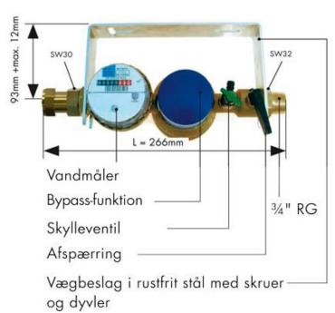
Vandmåler = Water meter Bypass-funktion = Bypass function Skylleventil = Flush valve Afspærring = Shut-off
