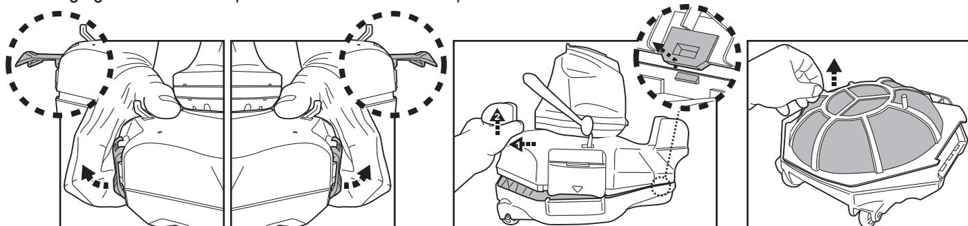
2. Detach the filter cover and remove the debris from the compartment. It is recommended to clean the filter cover net with splashing water. If brushing is deemed necessary, use only a soft brush to clean it carefully and gently to avoid damages.
