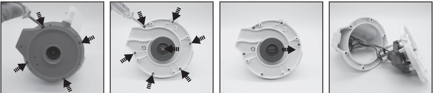
3. Remove out the battery pack to expose the PCBA. To detach the battery connection wire, press on the clip of the connector to pull it out. **NOTE:** Wrap the connector immediately with insulating tape in order to avoid any short circuit caused by the contact of both wire terminals.
