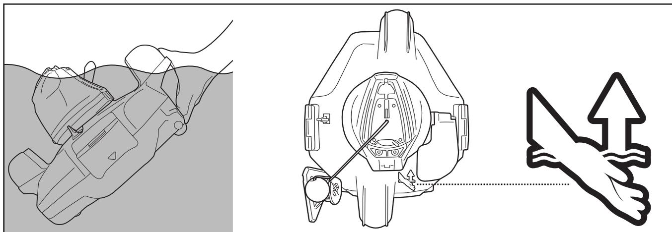
5. Slide the power switch OFF. Rinse the robot with fresh water after every use. DO NOT use any detergent.
