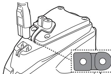
3. Connect the external adaptor to the power source. The indicator light on the external adaptor turns red once the charging begins. The indicator light on the external adaptor will turn green when the robot is charged.
