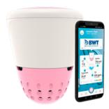
The BWT Pearl Water Manager is a digital pool water tester measures pH value, temperature, conductivity, and redox potential in both classic chlorine and saltwater pools in real time. The pool buoy is controlled via the associated BWT Pearl Water Manager app, which incorporates local weather data into the chemical dosing recommendations.
