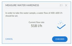
To determine the water hardness, the water sample should be taken at the nearest sampling point at a volume flow rate of 400-600 l/h.
