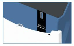
The maximum level of 100% in the multi-info touch display corresponds to a regenerative filling level of approx. 46 cm in the regenerative container.
