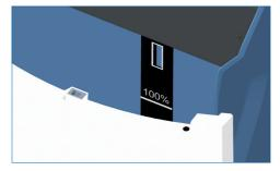
The maximum level of 100% in the multi-info touch display corresponds to a regenerative filling level of approx. 46 cm in the regenerative container.
