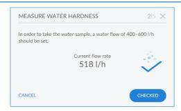
For determining the water hardness, the water sample should be taken at the nearest sampling point at a flow rate of 400 to 600 l/h.
