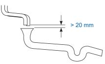
In accordance with EN 1717, the rinsing water and overflow hoses must be connected to the sewage system at least 20 mm above the highest possible waste water level (unimpeded drainage).
