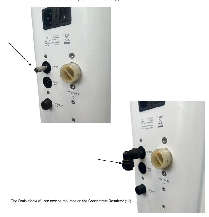
Cut the 8mm hose (6) in the needed length for connecting the unit to the Siphon (19). Push the 8mm hose (6) into the drain elbow (5).
