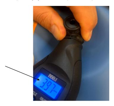
The factory default pressure aprox. 4 bars. The tank must be deflated to 1 bar.
