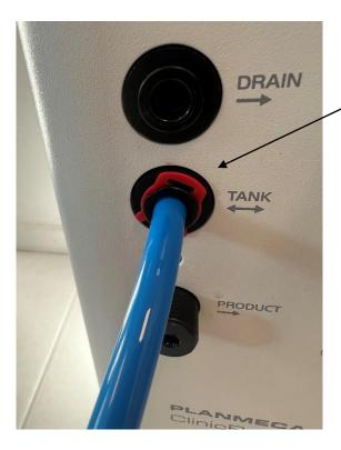
Mount the Female adaptor 8mm (20) to the pressure tanks (14) inlet. Push the 8mm hose (7) into the adaptor (20) and remember to lock it with a locking clip (13).
