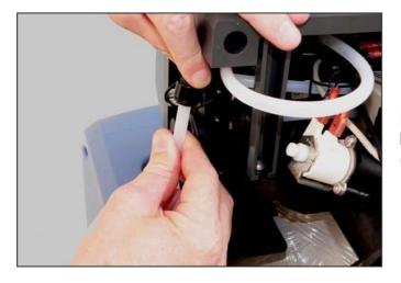
Run the the brine hose from the inside though the bore to the outside and insert it as far as it will go (a depth of about 15 mm) in the connection angle.
