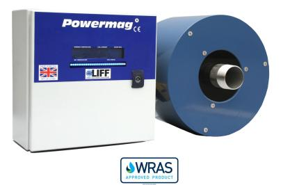
An electromagnetic physical water conditioner uses the principles of magnetism to inhibit formations of hard crystalline scale within hot and cold water services. The Powermag sets up a specific magnetic field which has an effect on the hardness salts within the water. This helps to inhibit and remove existing formations of scale, providing an environmentally friendly method of scale control without the use of chemicals
