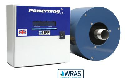
An electromagnetic physical water conditioner uses the principles of magnetism to inhibit formations of hard crystalline scale within hot and cold water services. The Powermag sets up a specific magnetic field which has an effect on the hardness salts within the water. This helps to inhibit and remove existing formations of scale, providing an environmentally friendly method of scale control without the use of chemicals
