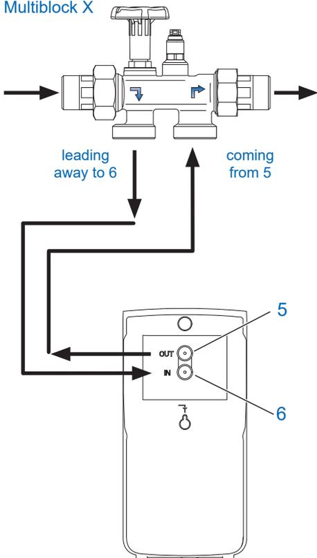
Connect the product as shown in the diagram opposite. A bypass is integrated into Multiblock X. The unit can be installed in horizontal or vertical pipelines.
